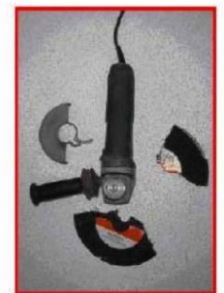
Angle grinder and disintegrated disk
