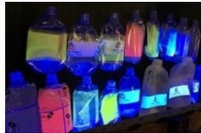
Chemical tracers are applied to the shrink label or plastic object and can be detected under UV lighting
